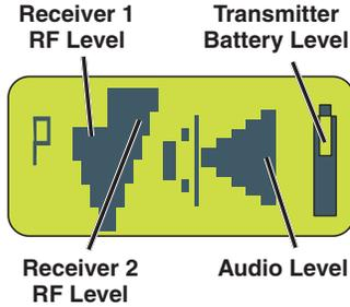
**NOTE:** When RATIO DIVERSITY is enabled, both receivers are combined to pick up the same transmitter, so the Main Window will display a single audio channel as shown here.
