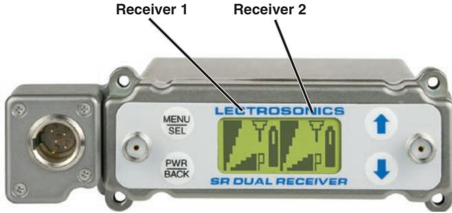
The control panel is a rugged, dust and water resistant design with membrane switches for the control interface. A backlit, graphics-type LCD is used to set up and monitor the receiver. Navigation through the menus is straightforward with text prompts for value and mode selections. The Main Window shown here is used during operation to display RF and audio levels, transmitter battery status, pilot tone status and diversity activity for both receivers.
