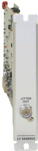
This unit displays eye patterns. It is installed in a LV 5800 input slot. By combining with the LV 5800 input unit, eye pattern waveforms of SDI signals can be monitored. Automatic measurement of parameters such as amplitude, rise time, and fall time is also possible.
