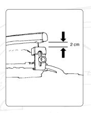
Fig. 5 Leave a gap of approx. 2 cm (1 inch) between the camera and the support arm.
