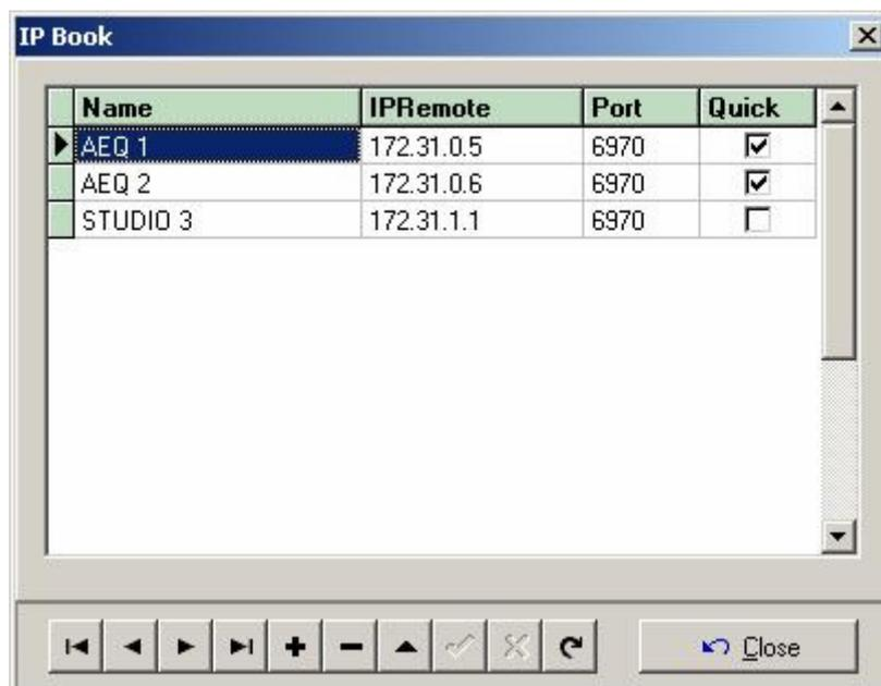
To enter a record in the IP book, you must type in the name, IP address and port directly over the fields. To enter a new record, just press the '+' button, and to delete one, use the '-' button.
