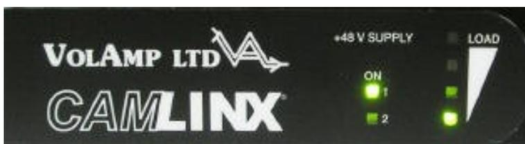
The Camlinx™ power link operates at 48 volts DC. The power comes from 48 volt supply in the base station, and is converted down to 12 volts at the head. Up to 60 watts (5 Amps) can be supplied to a Camera, over a distance of up to
