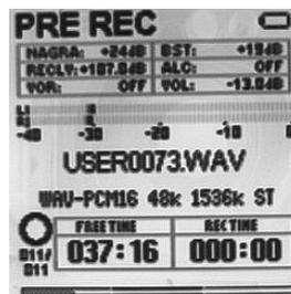
In this mode, the recording level can be adjusted in 0.5 dB steps using the " $\triangleleft$ " or " $\triangleright$ " keys: the value is shown in the window that appears. Initially, the value corresponds to the preset value stored along in the input device template. When internal microphone ("INT MIC") is selected, the recording level can not be adjusted.
