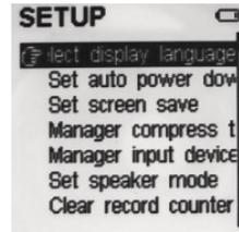
The “**SETUP**” menu gives access to several sub-menus. The most important are the compress templates creation and the input devices manager.
